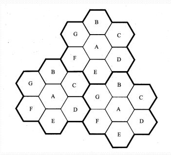
•In mobile-telephone nets these cells are usually hexagonal.
